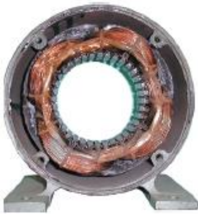
(c) running winding and starting winding 運轉繞組與啟動繞組
